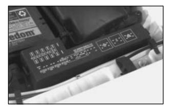
The engine compartment fuse block is located on the driver's side of the engine compartment. Lift off the cover to check the fuses.
